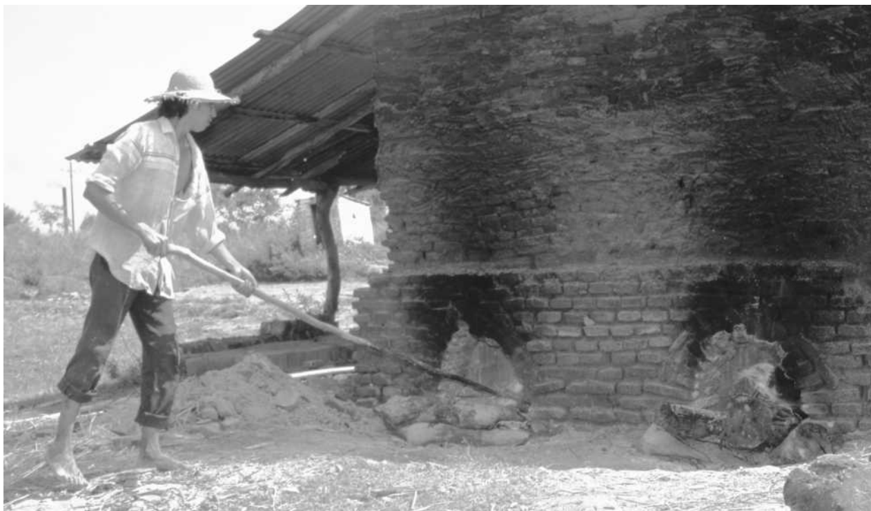
A brick kiln. The towns of Aregua and Tobatí both produce ceramic and clay work.
